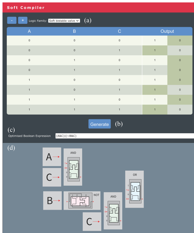
Fig. 1. The web-interface of the Soft Compiler. (a) The user defines the number of inputs to the soft circuit, the soft logic family (here: “Soft bistable valve”) and a truth table, mapping input combinations to a desired output response. (b) Once the truth table is defined, “Generate” executes the compiler and outputs (c) an optimized Boolean expression, and (d) a schematic depicting the optimal wiring configuration that the user then implements during circuit assembly.
