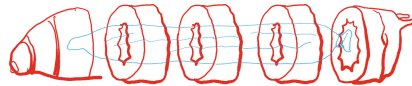
Fig. 2. Sketch of the soft maggot robot. A central bag of fluid is surrounded by muscle segments.
